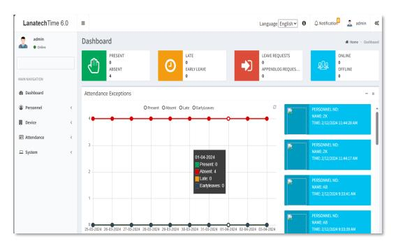
On the main interface, four menu panels are displayed: *Personnel, Device, Attendance,* and *system*. Click a related following function below any panel to quickly access the corresponding interface.
